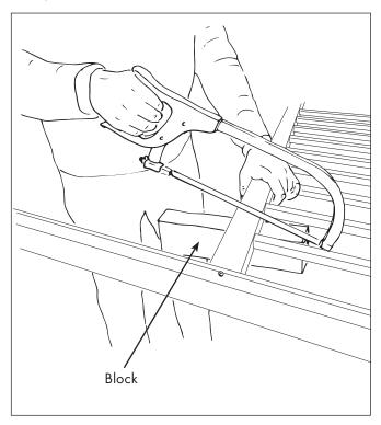
Step 4 - Cut through the bottom rail in the same way as the previous step.
