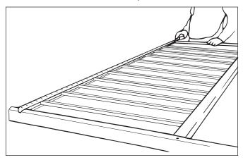
Step 3 - Place a block under the top rail and cut through using a hacksaw with a fine tooth blade. If you have difficulty with the pool channel (with the square holes) cut it using tin snips.
